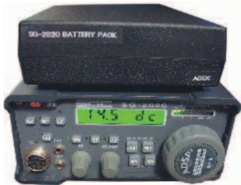
Figure 5—The battery pack and the transceiver. The pack furnishes sufficient voltage for over 1½ hours of operation at the 20 W level. Note the output voltage of the battery pack; the SG-2020 can meter the dc input voltage on its display.
